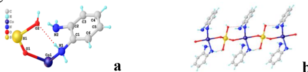
Figure 1. Molecular structure of the polymer complex [Co(C 6 H 4 (NH 2 ) 2 SO 4 ) n ] (a,b)
