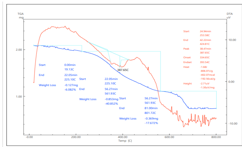
Figure 1. Derivatogram of alkyd enamel sample PF-115 with the addition of cobalt-magnesium-containing phthalocyanine (Co-MgPc) pigment
